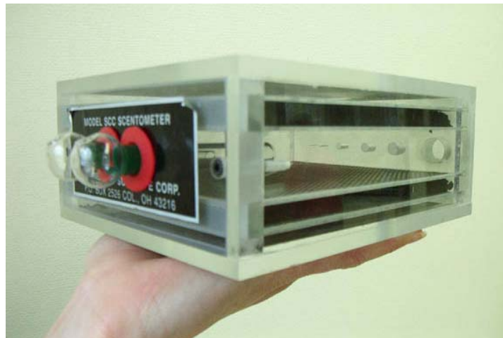
Figure 2. The Scentometer Field Olfactometer (Barnebey Sutcliffe Corp.). Note the two glass nostril ports to the left and the series of orifice holes at the back of the unit to the right in this photo.
