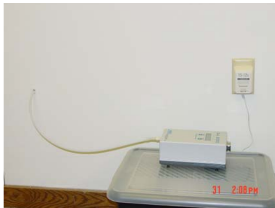
Figure 4. Advanced Calibration Designs, Inc. Cal2000 Hydrogen Sulfide Gas Generator. The gas feed line travels from the generator through the chamber wall to the injection point.
