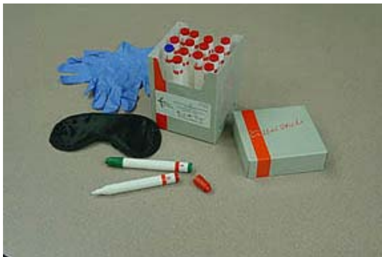
Figure 1. The St. Croix Sensory Odor Pen Kit. Included in the picture are the blindfold, non-latex gloves and the set of 14 n-butanol pens (red) and odorless blank pens.
