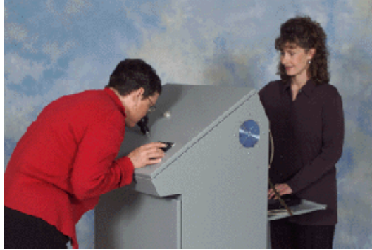
Figure 1. AC'SCENT Olfactometer (St. Croix Sensory) showing assessor sniffing on the left side while a laboratory technician is monitoring the test on the right.
