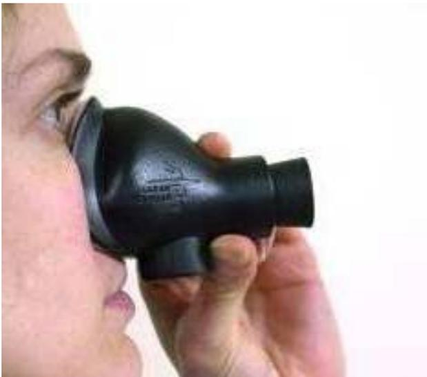
**With the stopper in place (LEAK TEST), you should not be able to inhale through your nose.**
