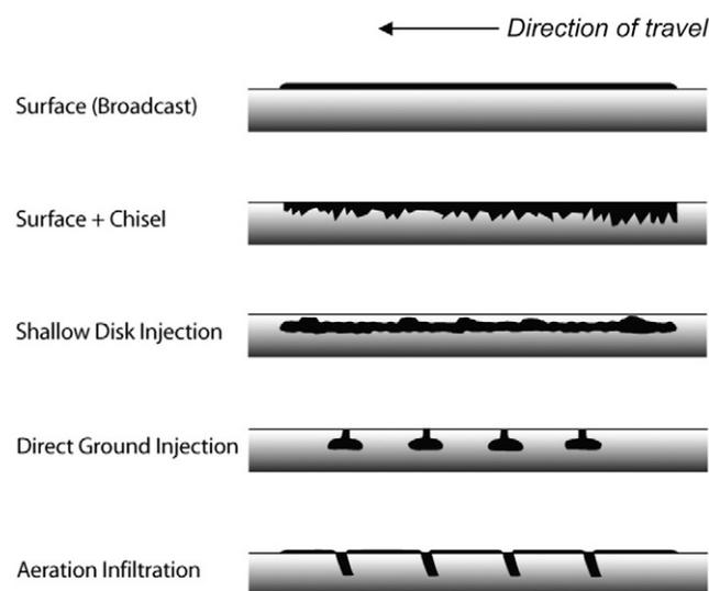
**Fig. 1. Schematic of manure distribution for the various field application methods.**
